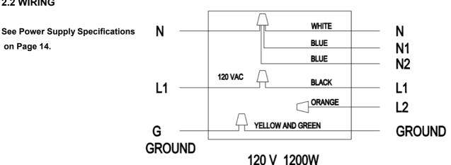
IF THE APPLIANCE IS TO BE HARD WIRED IN, THE POWER CORD MUST BE **REMOVED (SEE INSTRUCTION #1 ON PAGE 20)**
