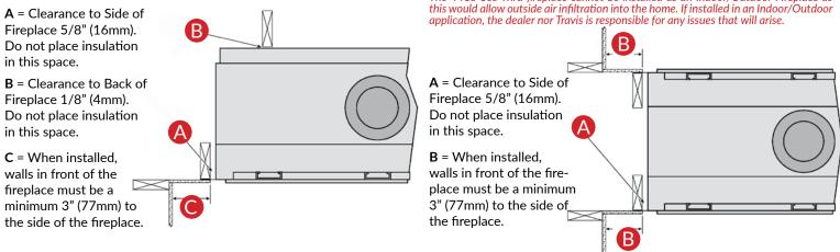
NOTE: ALWAYS REFER TO THE PRODUCT OWNER'S MANUAL FOR COMPLETE INSTALLATION INSTRUCTIONS. FAILURE TO DO SO CAN RE-SULT IN VOIDING OF THE WARRANTY AND PRESENT A POTENTIAL SAFETY HAZARD! MANUAL CAN BE FOUND AT WWW.FIREPLACEX.COM
