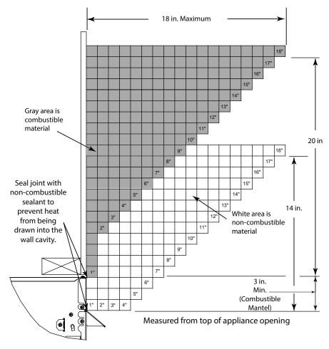
Note: Reducing clearances further requires non-combustible construction materials (eg: steel studs, durock, etc) to a height of 12 inches above the framing height.
