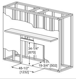
NOTE: Add 1/2" to width and 1/4" to height dimensions when using optional trim kit to finish the installation of a custom cabinet, mantel or other built-in enclosure.
