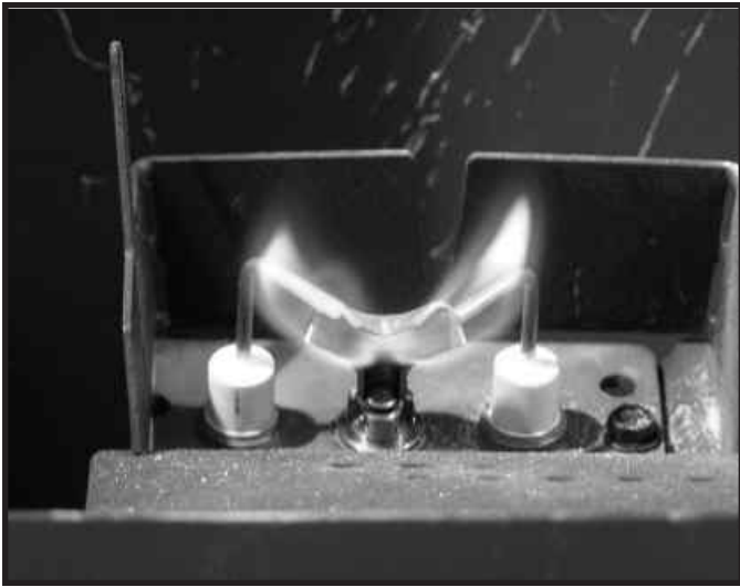
Figure 4.2 IPI Pilot Flame Patterns - Generic Pilot Bracket Shown
