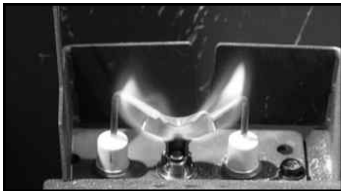
Figure 4.2 IPI Pilot Flame Patterns
